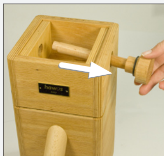
Figure 5 Pull the adjusting wheel together with its axle out of the side.
