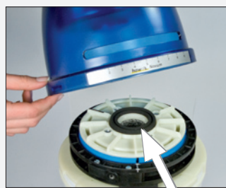
Figure 4 Make sure that the foam rubber gasket is properly seated (arrow). Mount the funnel and secure with the funnel bracket screw and adjusting lever.
